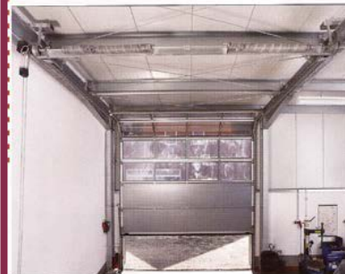
Sectional door SLUV, low headroom fitting with rear spring shaft, for headroom requirement above 270 mm, and reduced sideroom requirement.
